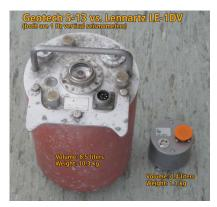
But using a modern electronically enhanced seismometer has more advantages: Each sensor is individually adjusted and calibrated to less than 1% deviation from the theoretical transfer function and transduction factor, so sensors are perfectly interchangeable without the need to keep track of which sensor was connected to which station at which time. Mechanical sensors have much greater parameter variance, both between individual instruments and over time.
